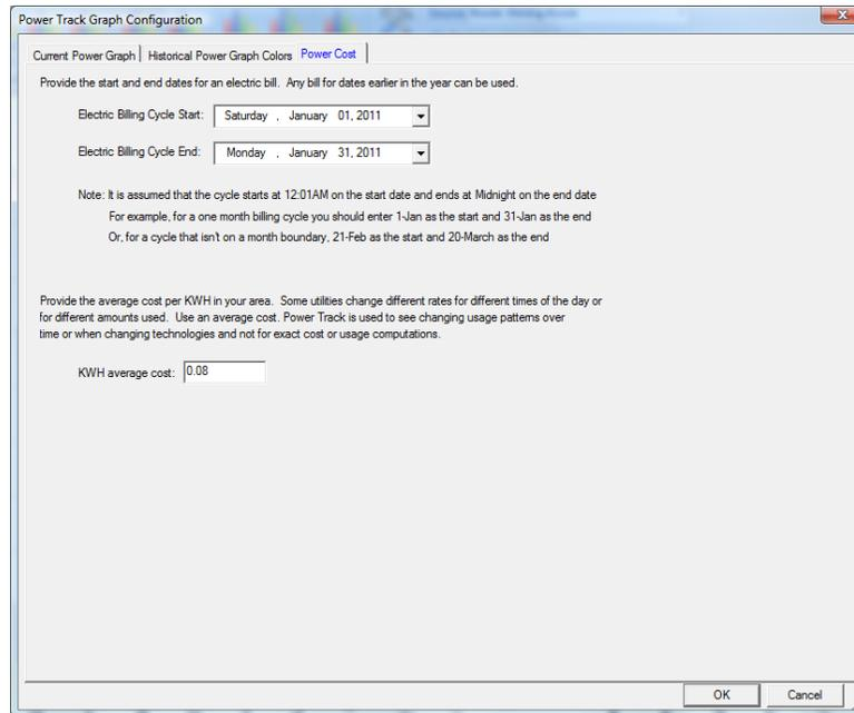
The power cost is at the bottom on the dialog. You can usually get this information from a power company bill. In some locations the power cost varies with time or day or usage over the billing cycle. In this case just enter an approximate average value. For these purposes this is sufficiently accurate.
