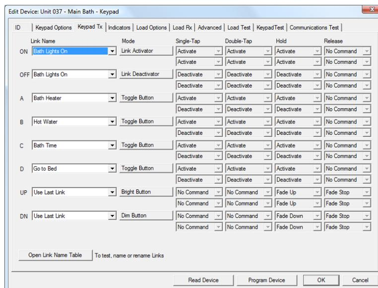
When HCA sees the “Bath Lights On” link being transmitted it “knows” that the load has been turned on and at what level.
