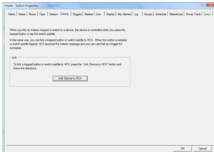
In the case of a KeypadLinc, you should link the “On” button to HCA.
