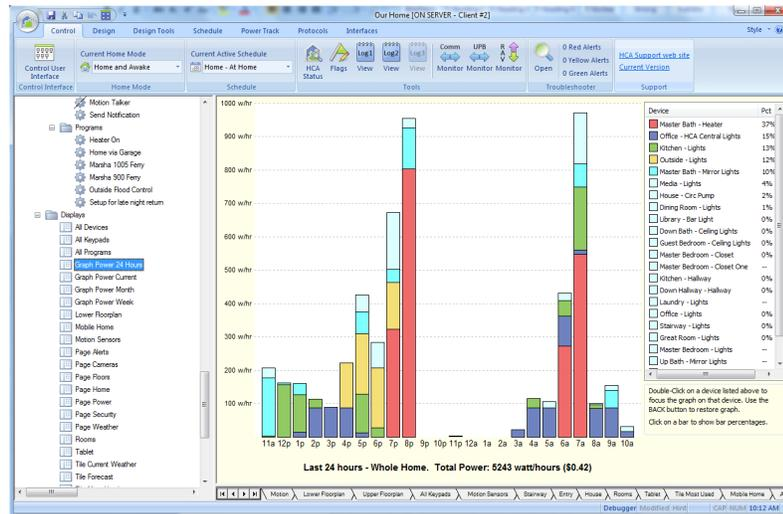
Unlike the current power graph where colors are assigned to individual devices or rooms, here colors used are to show the largest power users. These colors are selected from the Graph Setup dialog on the *Historical Power Graph Colors* tab.
