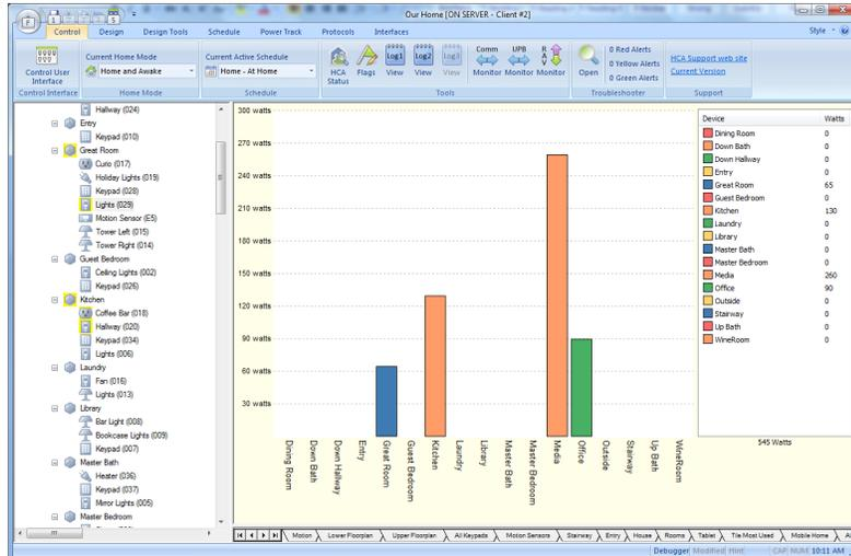
Each device or room shows as a bar representing the current power usage in watts. The list on the right shows the data in tabular form.
