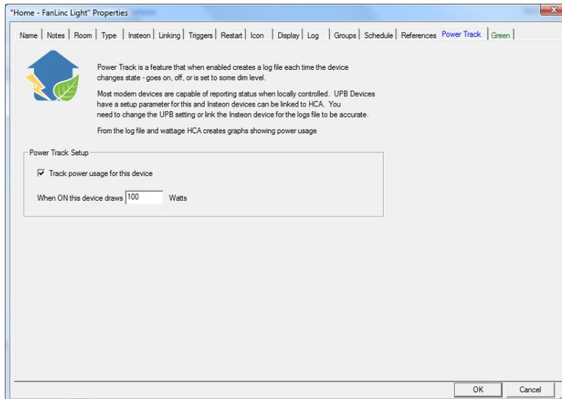
All you need do is to tick the checkbox and supply how much current the device draws when at full power. For lighting this is the bulb wattage. For appliances this is usually listed on a sticker someplace on the device.
