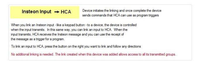
Once added to the design you can create program triggers for the events you want to handle. For example this program triggers on the message when the sensor detects that the window or door is open.
