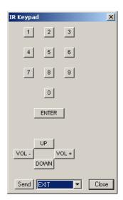
From the test keypad, pressing a button causes the IR sequence to be transmitted by the selected GC-100 out the selected port.
