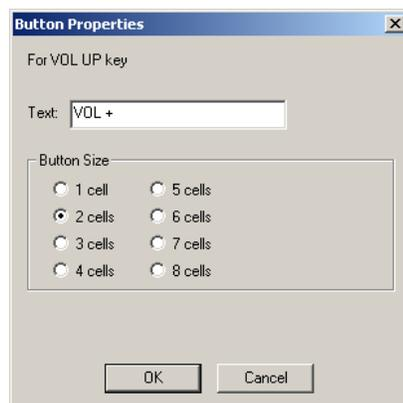
In the above example, several buttons have different names than listed in the keypad button list (Vol+ instead of Vol Up). This is because the name has been modified by opening the button properties and entering a new name.
