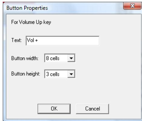
In the above example, several buttons have different names than listed in the list of possible keypad buttons (Vol+ instead of Volume Up). This is because the name has been modified by opening the button properties and entering a new name.
