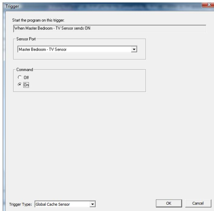
Select the GC-100 sensor and if the program should be triggered when the sensor sends an ON or an OFF.
