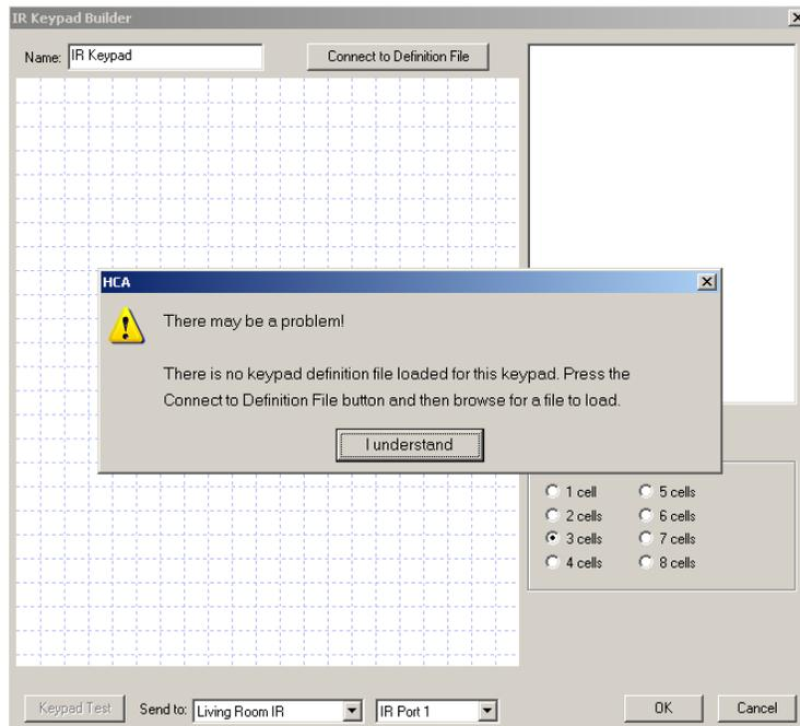
As the popup message points out, the first action you need perform is to connect this keypad to a definition file. Pressing the *Connect to Definition File* button displays this dialog. Press the *Browse* button to locate the IR definition file you created with the IR Learner.
