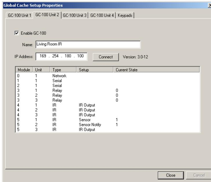
Configuration of the ports is done using the software from Global Caché or the internal web pages of the GC-100. While HCA can read out the setup it does not provide facilities to configure the ports.
