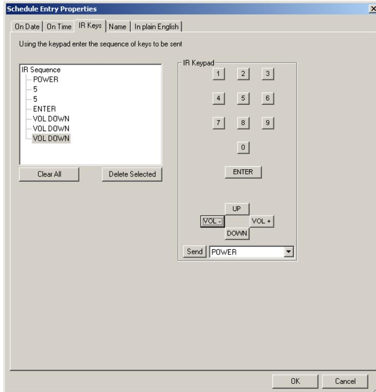
Enter the sequence you want to transmit in the same manner as the Visual Programmer. The final tab (or wizard step) of the schedule entry shows in text the sequence to be transmitted.
