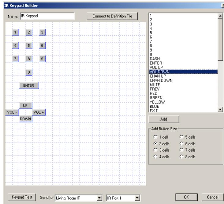
This dialog looks a bit like the Visual Programmer. On the canvas are placed the keypad buttons. In the upper right of the dialog is a list of all the IR keys from the definition file.
