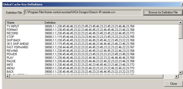
After the file is loaded, the key sequences display. Closing this dialog places you back in the Keypad Builder.
