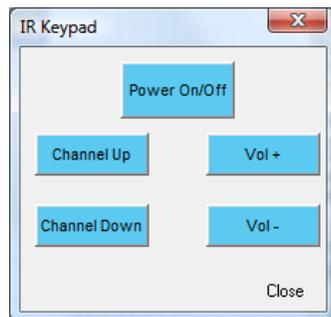
From the test keypad, pressing a button causes the IR sequence to be transmitted by the selected BC4 out the selected port.
