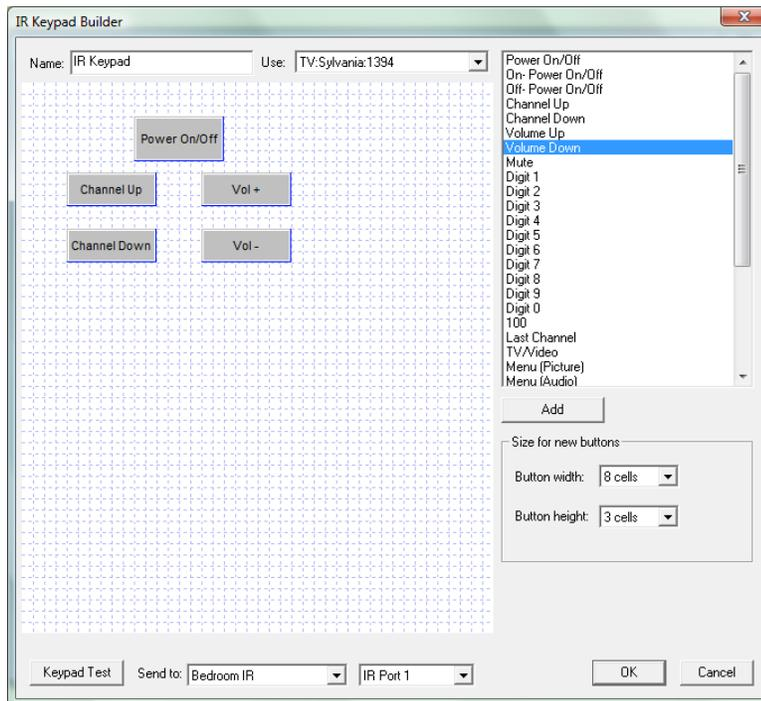
To add a new button to a keypad, select a key in the list of keys that performs the action that you want. Then select the button size and press Add, or like the Visual Programmer, select the key in the list and drag it on to the canvas.
