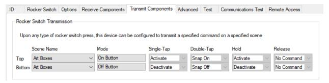
When in your home and you tap the top of the switch paddle, the load is controlled to ON – that's how the switch is electrically wired - and a scene activate command is transmitted as well. In this example, the scene named "Art boxes".
