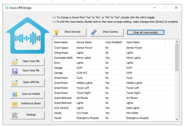
In the configuration software press the *Show Scenes* button. As described in the previous step, the list is organized by the controller of the scene. In the same way as devices, you can double-click on the "Yes" or "No" text to enable or disable voice support and double-click on the voice name to change.
