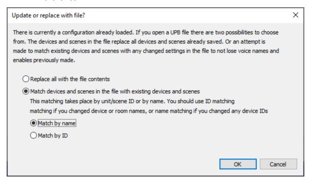
A final point on this: If you make a minor change in Upstart you <u>don't</u> need to reload the UPB file into the configuration program again. What's a minor change? Changing a preset level within an existing scene. If you do add a new device or scene, or add or remove a device from a scene, then you should reload your UPB file. But as said above, you will not lose any of your work in assigning voice names.
