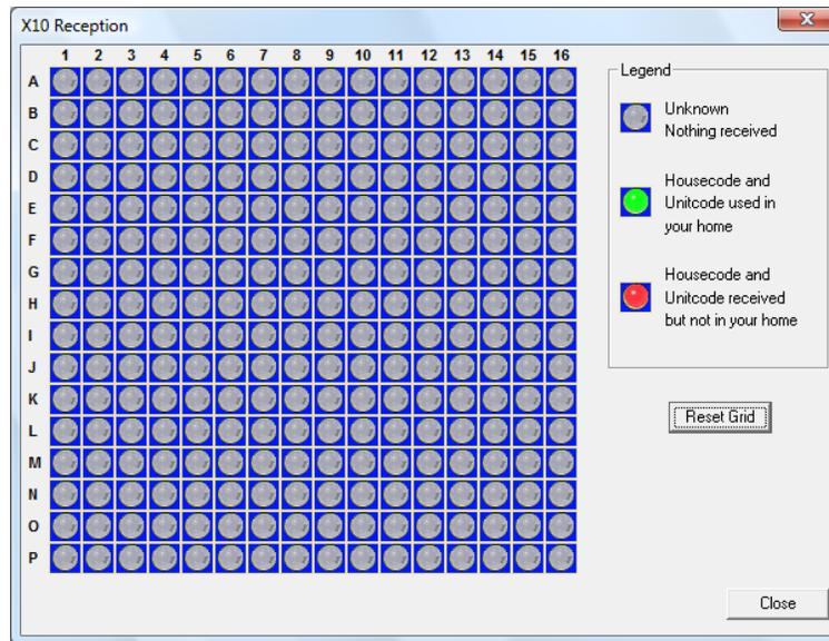
The large grid that appears in this tab shows, for each housecode and unitcode, if any X10 commands have been received by HCA and when. This could have been an ON, OFF, DIM or Status command.
