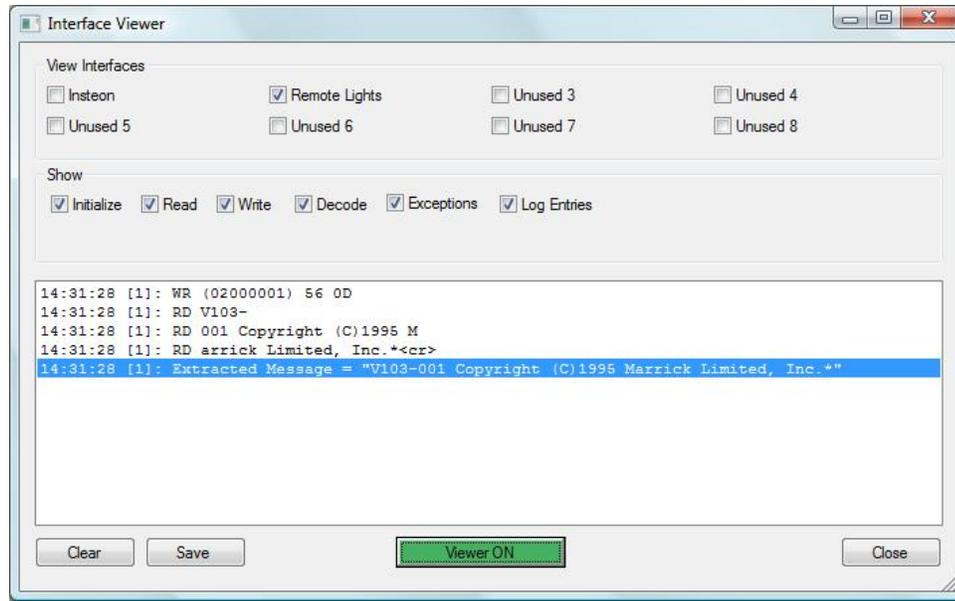
The names of the eight interfaces that can be configured are the first set of checkboxes. Tick the ones that you want to see data from. Interfaces not configured are listed as *Unused*.
