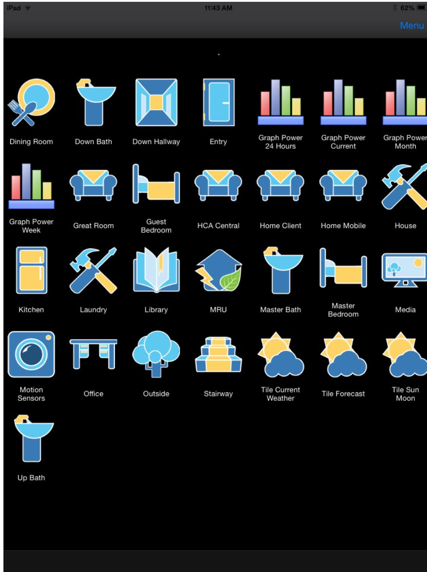
This example display, on an iPad mini, shows the familiar set of HCA icons. The same short and long taps on an icon like the other clients are implemented. To toggle the status of a device, a short tap toggles its state. Long taps are a bit different than the HCA Windows client and HCA Android client as the popup display doesn't appear until you release the tap.
