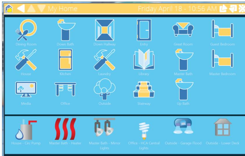
Like the Control User Interface, the same short and long tab methods are used to control a device, program, or group. Also, like the Control User Interface, the status bar color reflects the Alert level – red, yellow, or green, and the HCA icon used at the left end of the status bar changes color to show the home mode.
