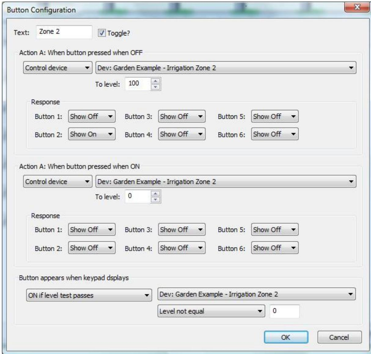
In this example, the first press of the key turns the selected device ON – to 100% - and the second press turns it OFF – to 0%.
