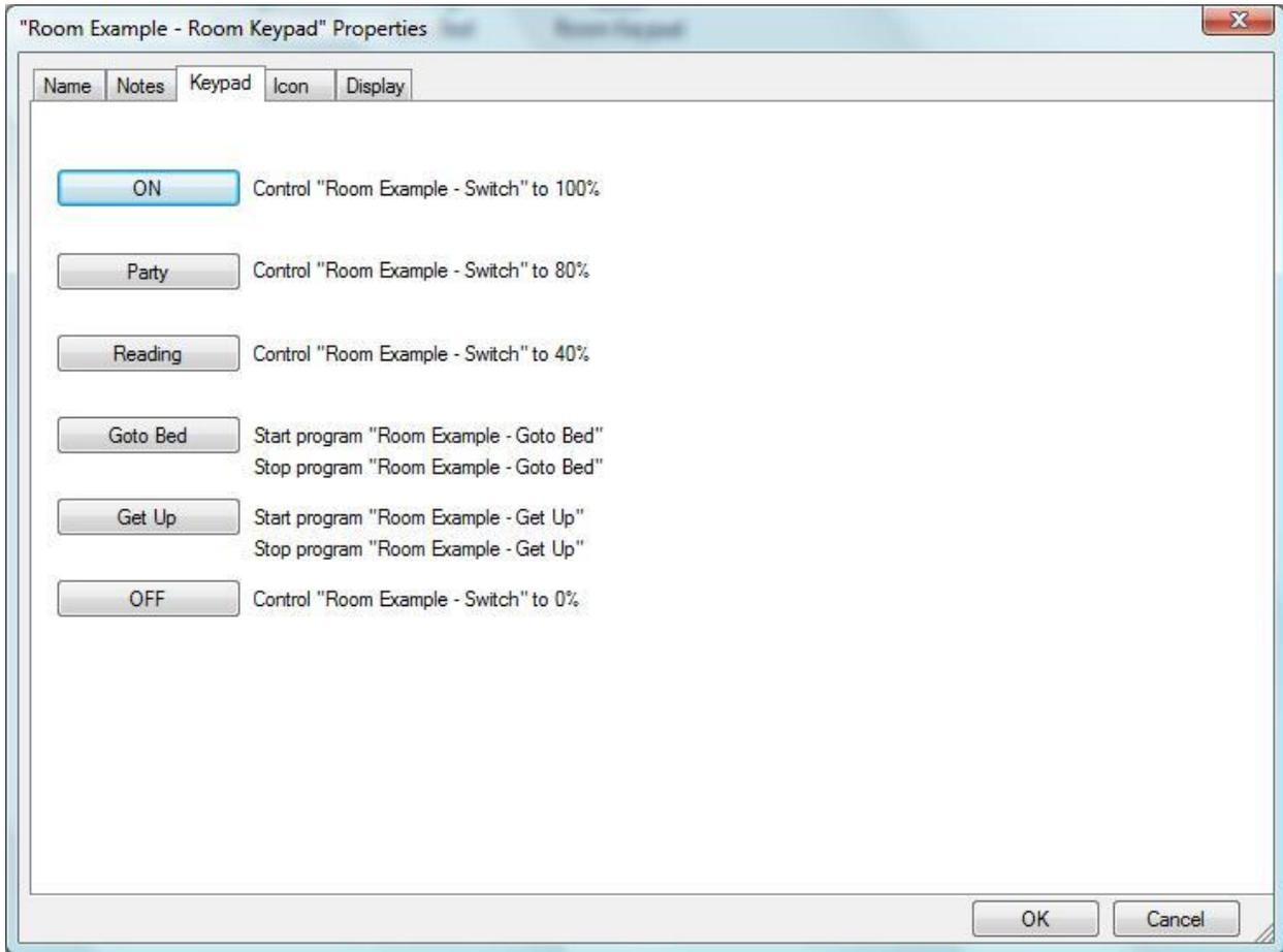
Note that keypads always have 6 buttons. In this example buttons 1, 2, 3, and 6 are not toggling buttons. Buttons that don't toggle perform the same action each time they are pressed. Buttons 4 and 5 are toggle buttons.
