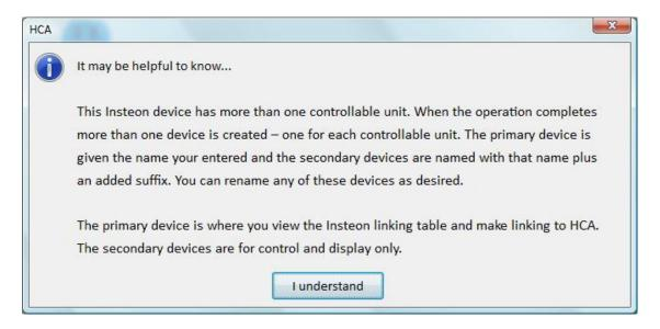
As explained above, six devices are created. The device for first sensor input is the "primary' device and the others are "secondary" devices. The sensor inputs can be used to trigger HCA programs or can be tested in programs. The output devices can be used in schedules or programs to control the relay.
