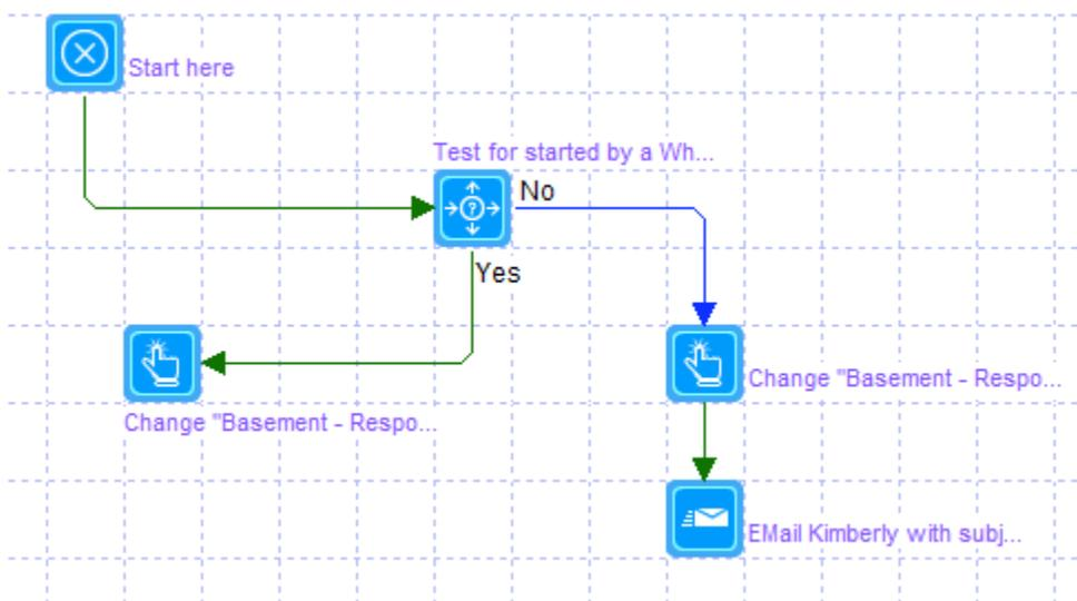
The actions of the program are to check the starting trigger and then change the program icon and its label to show if the water is ON or OFF.
