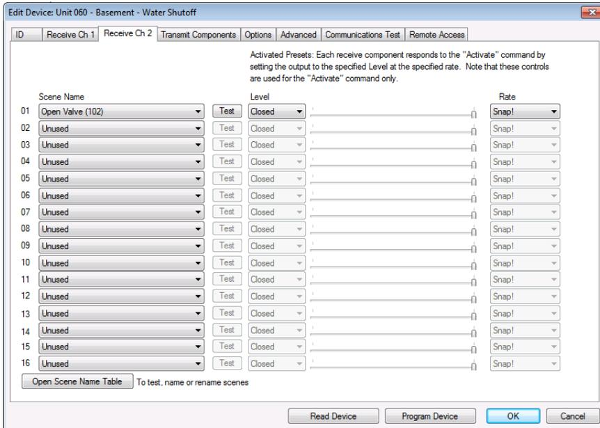
Once the two receive channels are configured then scenes are created to report when the valve opens and closes. These are assigned to inputs 2 and 3 on the module. The Simply Automated input module has documentation on how to connect wires to pins. Just use the “pin to pin” table given above to make the correct connections to what the WaterCop provides.
