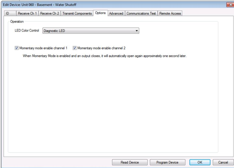
When HCA imports the UPB Network it creates devices for each of the inputs and outputs that the module has. On the “Remote Access” tab are where you choose which of the inputs and outputs you want HCA to create devices for, what they should be called, and what icons are used.
