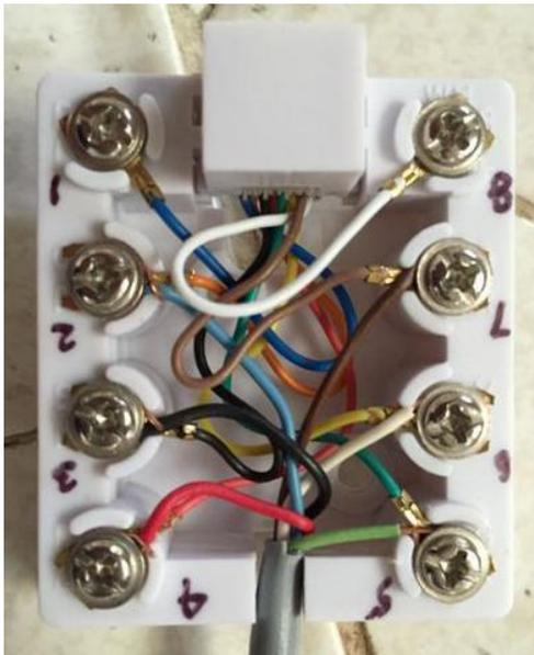
A terminal block with an RJ-45 jack provides a convenient way to connect the UPB module terminals to the RJ-45 connector on the WaterCop using an ordinary Ethernet cable as shown in this photo.
