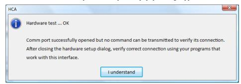
As the dialog says, the only test performed is that the serial port can be opened. There doesn't even have to be an actual interface connected to that serial port for the test to pass.
