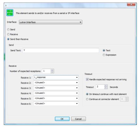
Select from the interface dropdown the name of the interface to use and then choose the option for send, receive, or send then receive.
