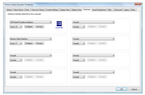
Choose "Generic Serial Interface" as the interface type, select the serial port to use, and press the *Connect* button. If the serial port can be opened a popup message appears:
