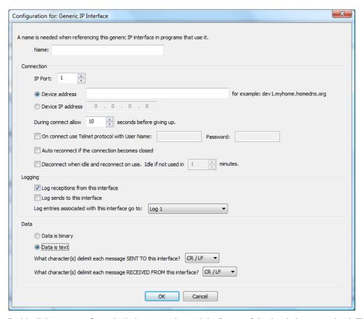
In this dialog you configure both the connection and the format of the data being transmitted. The data type – binary or text – and all the options for them are the same as in the generic serial interface.
