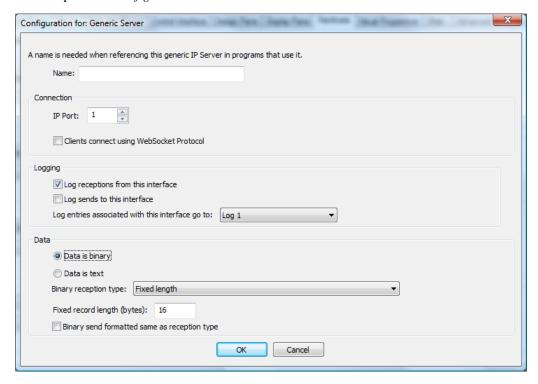
The main parameter is the port number. This port number must **not** be the port number the HCA Server uses and HCA clients – and mobile applications – connect to.
