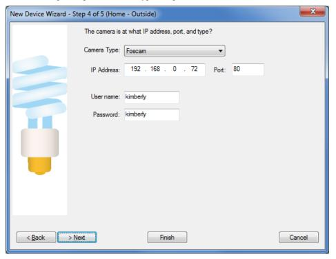
The camera type specifies what command set the camera uses. At this time the only selection is "Foscam".
